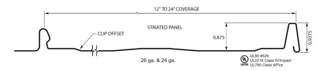
Standing Seam is an economical snap-together panel with a 1" standing seam for use over a solid deck. Panels are installed by using a pancake fastener in the panel's fastener flange. Available in 26 ga. and 24 ga. Minimum recommended slope is 3:12. Pan striations required for all 26 ga. panels.
